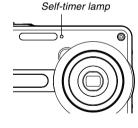
You can interrupt an ongoing self-timer countdown by pressing the shutter button while the self-timer lamp is flashing.
